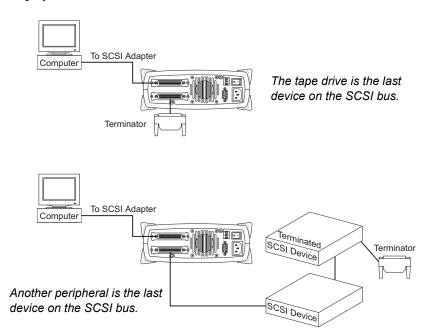
**Figure 2-7** Terminating the SCSI bus (external model)
